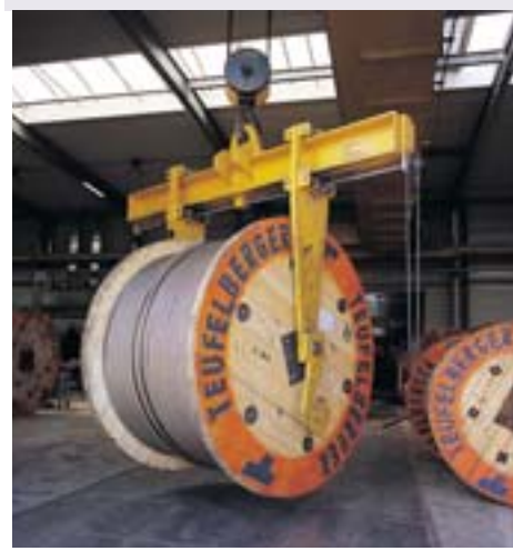
Lifting a reel with shaft inserted through centre hole
