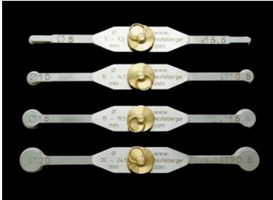
Measuring sheave groove with groove gauge
