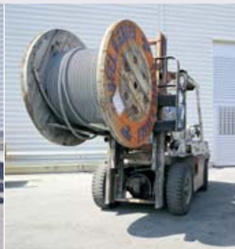
Lifting a reel with fork lift truck incorrect
